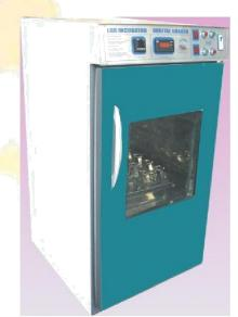
platform containing 16 flasks of 500 ml or 40 flasks of 100 ml or 34 flasks of 150 ml capacity is supplied with the unit as standard accessory
