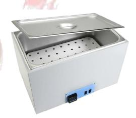
controller with an accuracy of  $\pm$  0.5°C . A high-speed stirrer is fitted to maintain temperature uniformity. The lid of bath is insulated, double walled fixed with hinges and is provided with locking arrangements along with capacity of 28/50/75ltrs (standard).
